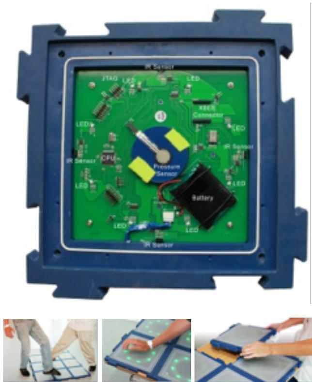
Figure E.2: Modular tiles used for feet or hand interaction.
