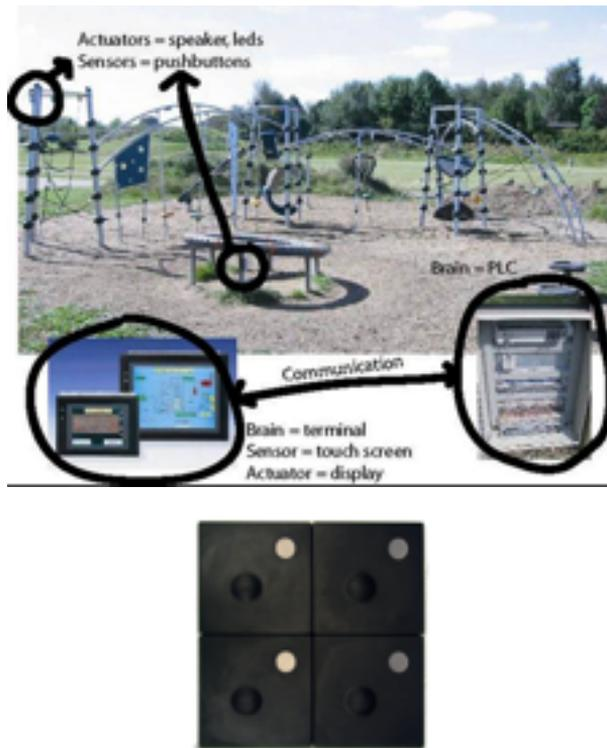
Figure E.1: Examples of mechatronic playgrounds. Left: sensors and actuators on a traditional playground product. Right: wire-connected, interactive tiles as floor surface for playgrounds.
